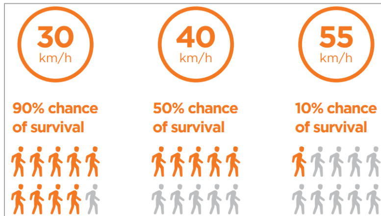
Figure 2: Vehicle speed and pedestrian crash severity - Vision Zero Surrey, 2019 Year in Review
